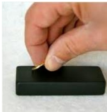
A touchstone - used for testing alloys of gold.
